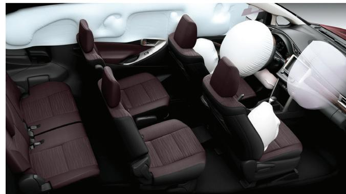
**7 SRS AIRBAGS** - Stay protected in all rows of seating with full wrap-around safety in the event of an impact.
