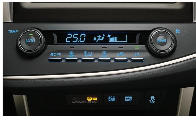
**AUTOMATIC CLIMATE CONTROL** - Take control and comfort to the next level with this feature. Adjust air level or speed from where you're seated, and turn it off and on as you please.
